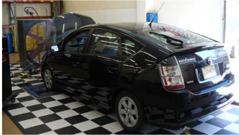
EPA testing procedures on a chasis dynamometer.
