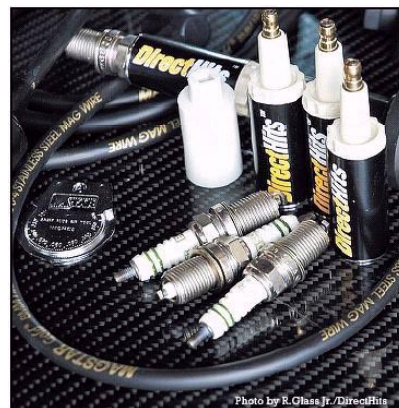
The DirectHits® capacitor mounts on a standard spark plug to boost spark energy.
